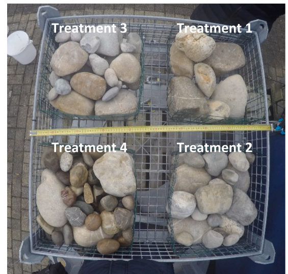
Fig. 2. The three stainless-steel units (1x1x1.4 m, left panel) used to test the effects of different habitat complexity treatments. The units were composed of a metal supporting structure and a one-by-one meter grid container of 20 cm height that was subdivided into four 45x45x20 cm compartments, allowing for 10 cm space between each compartment (right panel). The top of the table was covered by a 1x1m cover with a 2 × 2 cm mesh (not pictured here).
