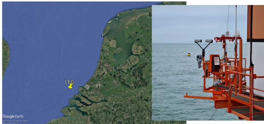
Figure 1. A map showing the location of the Lichteiland Goeree (LEG) platform, where concurrent rain and wind speed measurements were conducted (Caboni et al., 2024), and a picture of the OTT Parsivel 2 disdrometer installed on the platform are shown. Map courtesy of © Google Earth.
