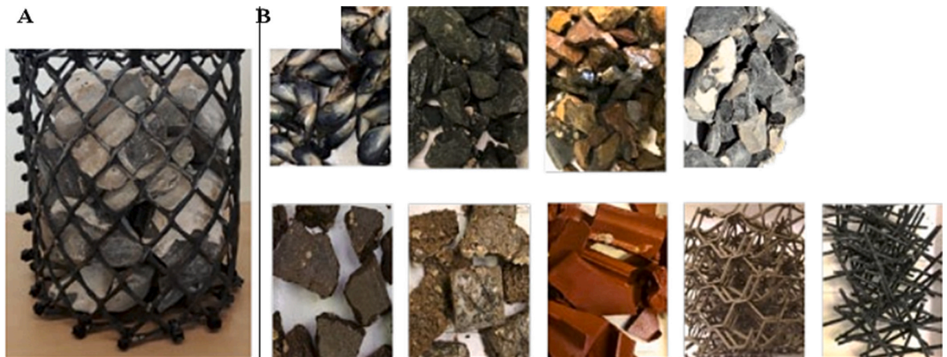
Fig. 1. A) basket used to hold the substrates, in this example filled with silex. B) overview of the different substrates used in the field experiments. From top left to bottom right: mussel shells, granite, sandstone, silex, concrete, EConcrete, roof tile, BESE, steel.
