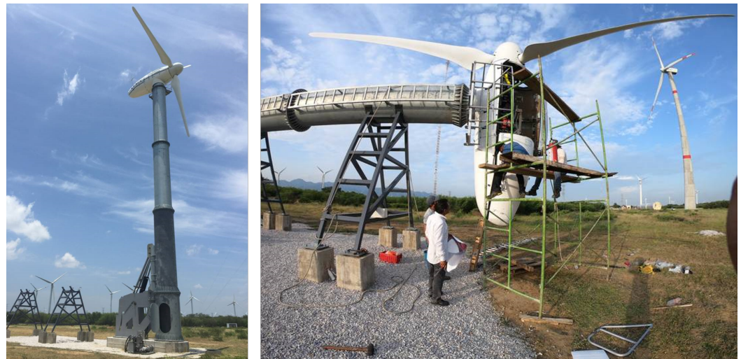
Figure 7. 30 kW collapsible turbine trials at the Regional Centre for Wind Energy Technology site in Oaxaca in 2019. Taken from Hernández-Arriaga [60].
