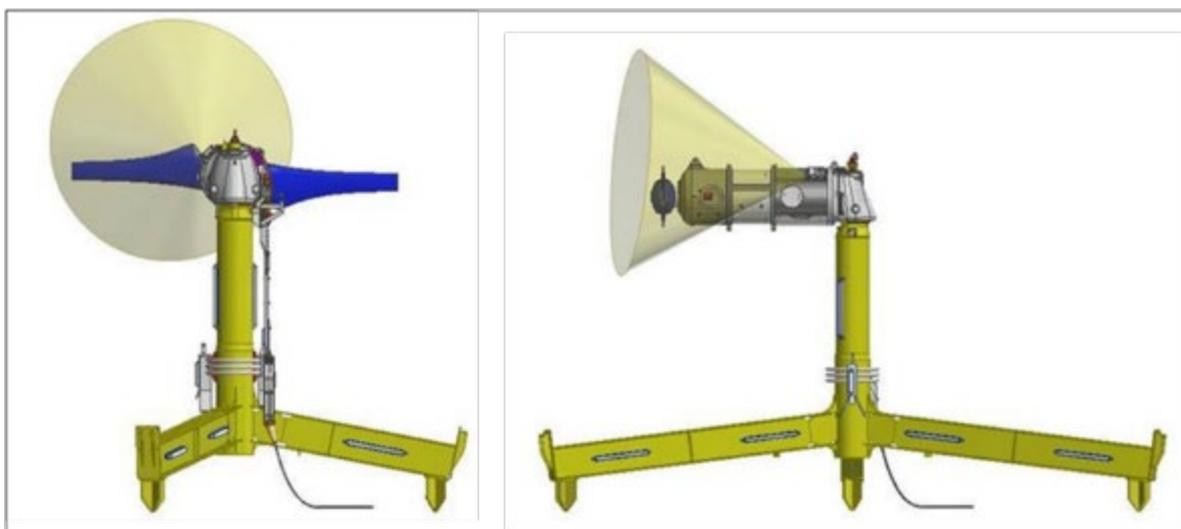
**Figure 5-2** Subsea camera system for turbines in the Shetland Tidal Array, showing field of view.
