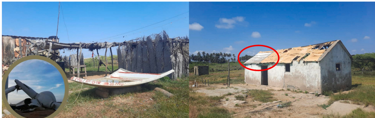
Fig. 7. Parts of the wind turbine are used as boats (left) and part of the fiberglass from the wind turbine propellers was used for the roof of a house (right). Source: (Rivero, 2024).
