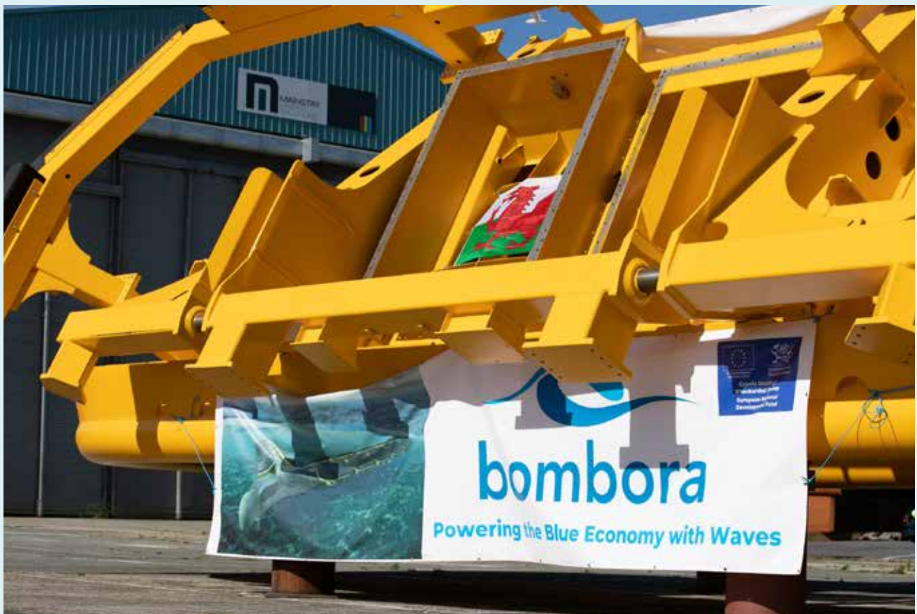
Bombora's full-scale 1.5 MW mWave prototype (Credit: Bombora Wavepower.)
