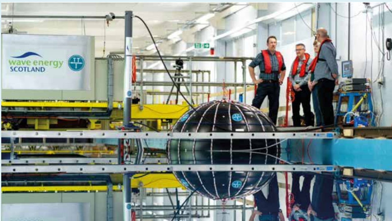
Testing of Tension Technology International's NetBuoy™, funded by WES (Credit: WES)
