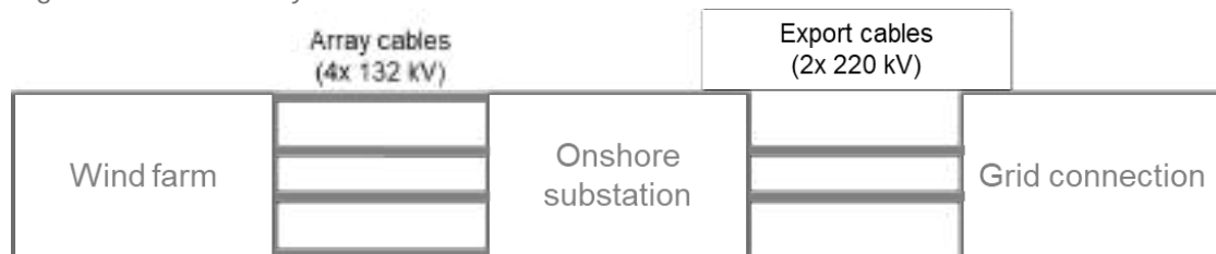
Figure 61 Electrical layout at Puttalam
