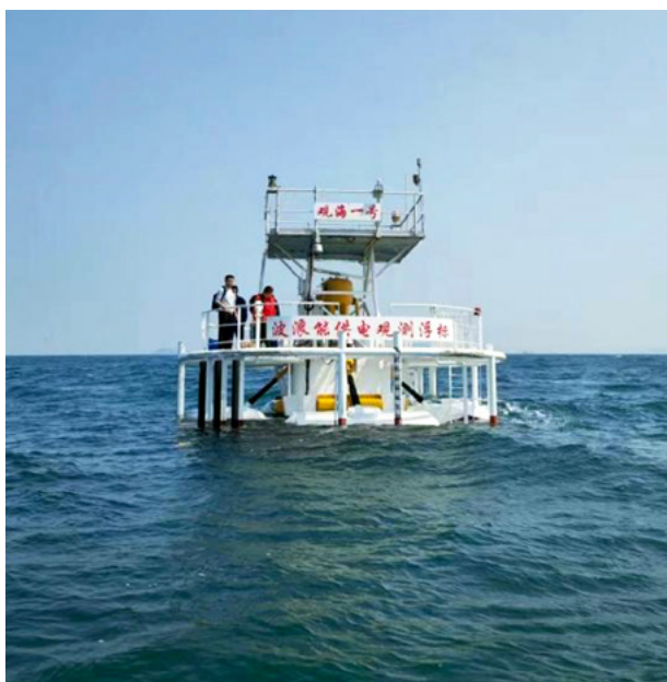
Guanhai I wave energy buoy in sea trial
