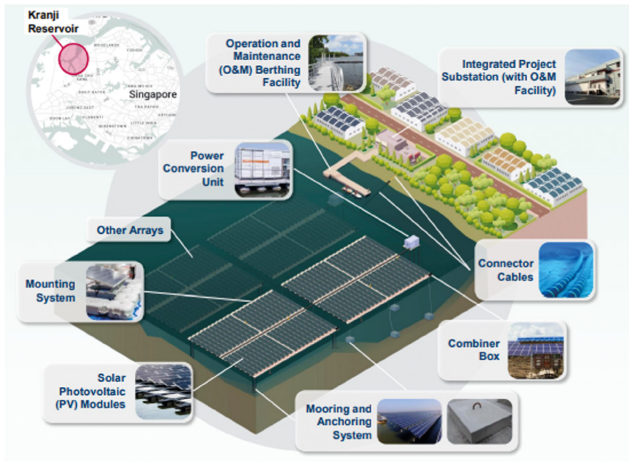
Figure 9: Floating Solar system planned in Kranji Reservoir
