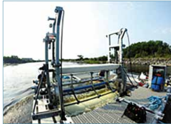
Floating ducted crossflow turbine (Mavi Innovations)
