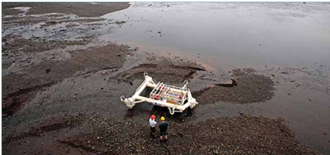
Fundy Advanced Sensor Technology (FAST) platform
