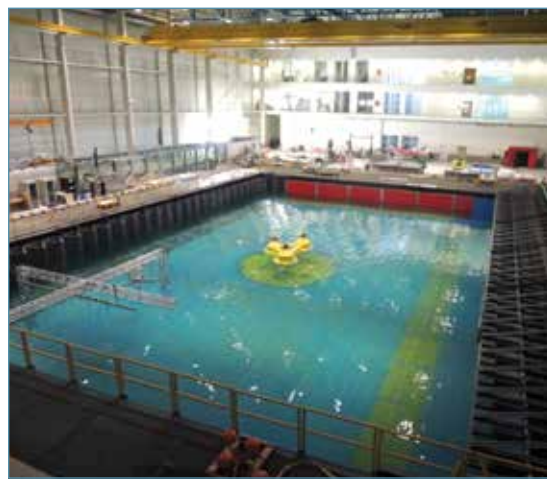
Tank testing campaign of the Undiplat's 1:20 scale prototype.
