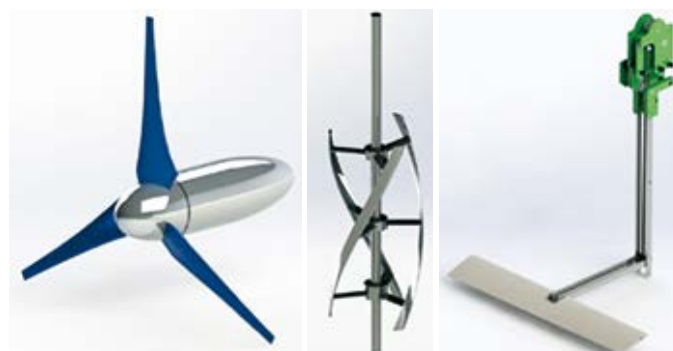
Active Control Tidal Turbines: Horizontal Axis, Vertical Axis, Flapping Hydrofoil
