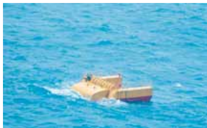
◀ Duck-2 wave energy device under testing
