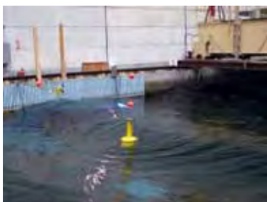
▲ Wave power generation experiment conducted in a wave tank (1/16) -Mitsui Engineering & Shipbuilding-
