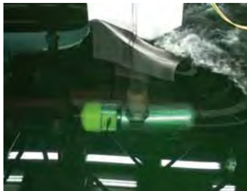
▼ Tidal power generation experiment conducted in a wave tank (1/10) -Kawasaki Heavy Industries, Ltd-
