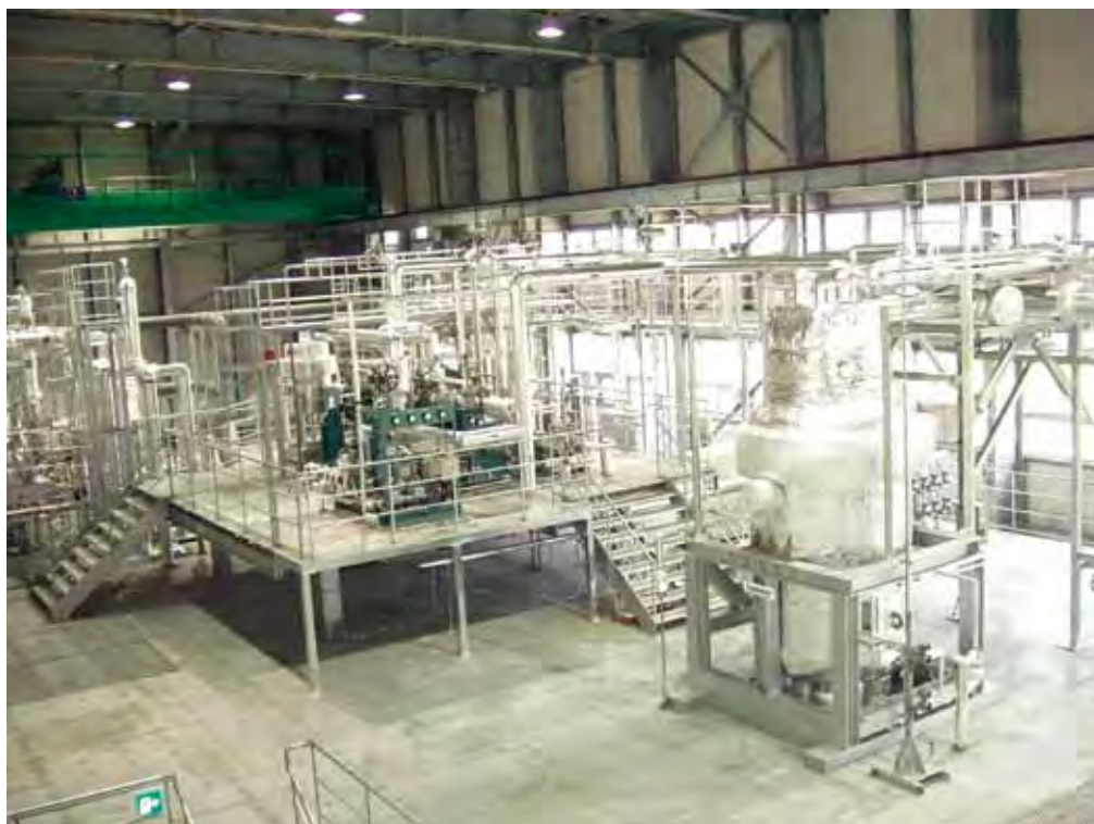
▲ 30kW OTEC system (Saga University)
