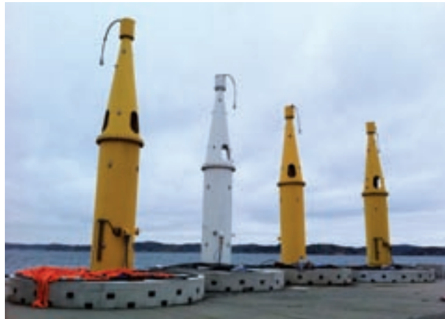
Linear generator-buoy units of Research Project for Wave Power – Lysekil Project
