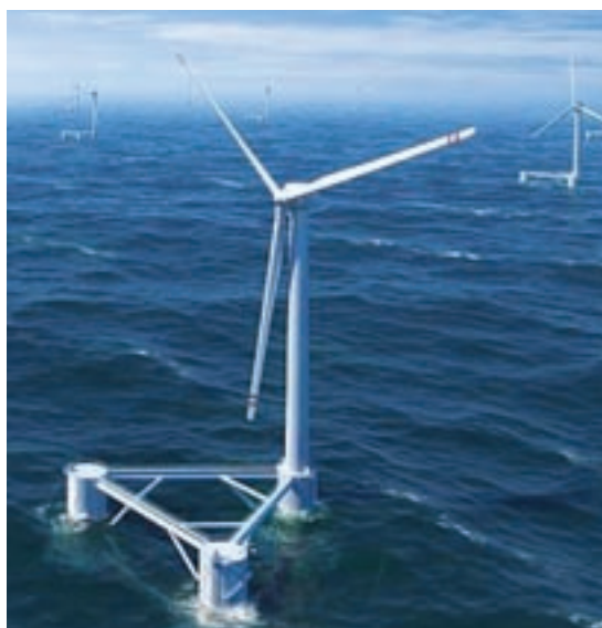
Figure 2: Artist's Impression Of Windfloat Concept: Various Technical Synergies With Wave Energy Devices (Picture Courtesy of Principle Power Inc.)
