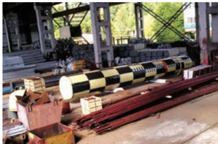
Experimental model in sea keeping basin with irregular waves and hull of FWEPS pilot module under manufacturing (yellow-black cylinder in the centre of picture)
