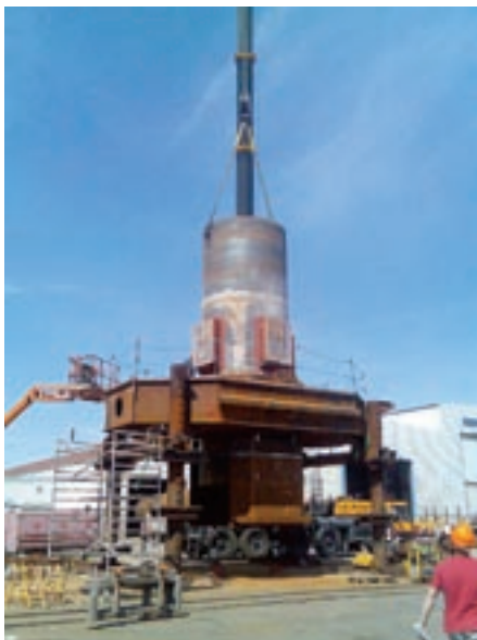
MCT SeaGen device – Pile and Collar
