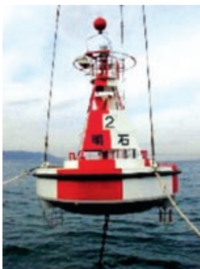
Navigation Buoy with Darrieus Turbine
