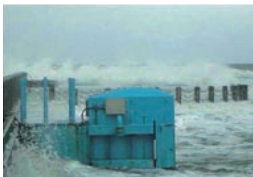
Demonstration test of OWC type wave energy converter in Niigata
