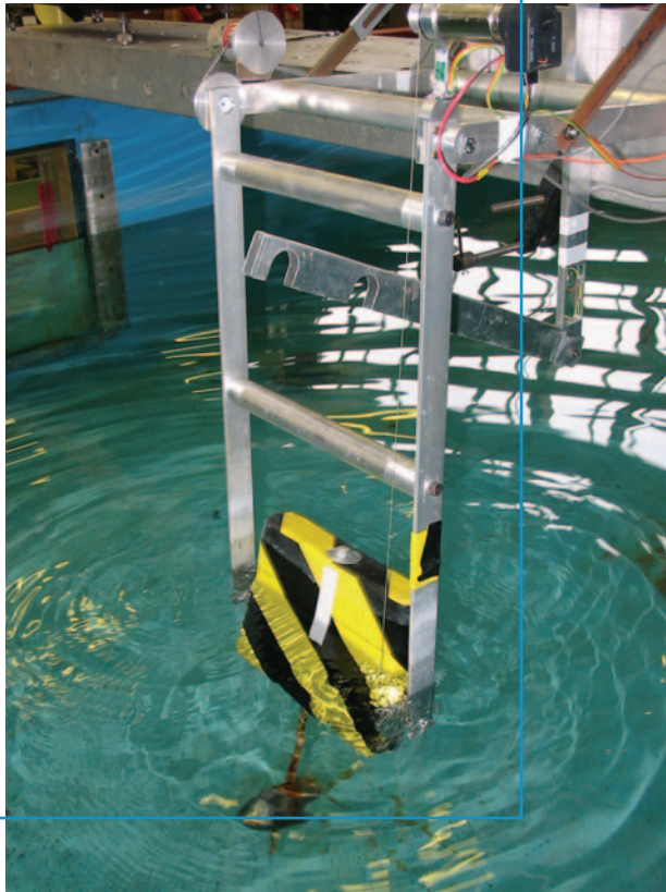
Figure 13 | Tank testing of the PS Frog Mk 5 (Lancaster University)
