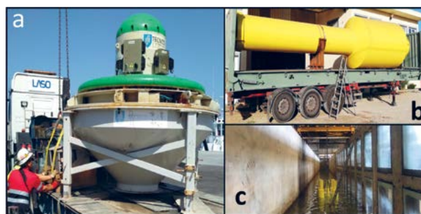
(a) Biradial air turbine after two years of sea trials in the Bay of Biscay, Northern Spain. (b) Wave-powered oceanographic buoy. (c) Model tests of wave-powered floating platform.
