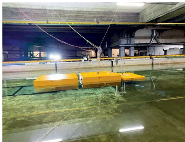
NEMOS designed WEC scale model at DST's wave tank (source: Space@Sea)
