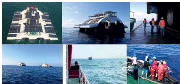
GIEC floating energy platform in open sea test (Installed wave energy 200kW, solar energy 60kW, a desalination facility with daily production of 6 tones water).
