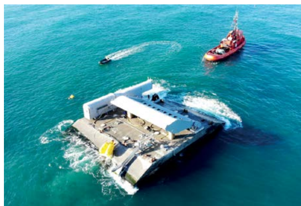
Deployment of the First-of-a-Kind (FOAK) WaveRoller (300 kW) offshore Peniche, Portugal
