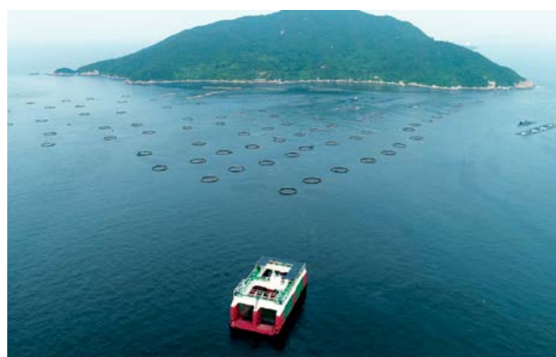
GIEC floating energy platform in open sea test (Installed wave energy 200kW, solar energy 60kW, a desalination facility with daily production of 6 tones water).
