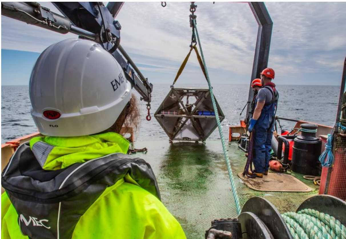
Figure 7 - ADCP recovery at EMEC
