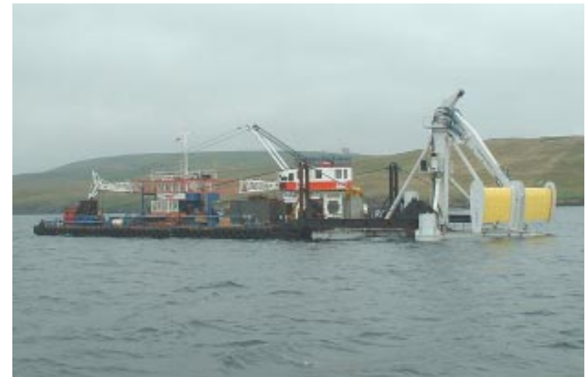
"Stingray" tidal current system in Yell Sound off the Shetland Islands (Courtesy of The Engineering Business, Ltd.)
