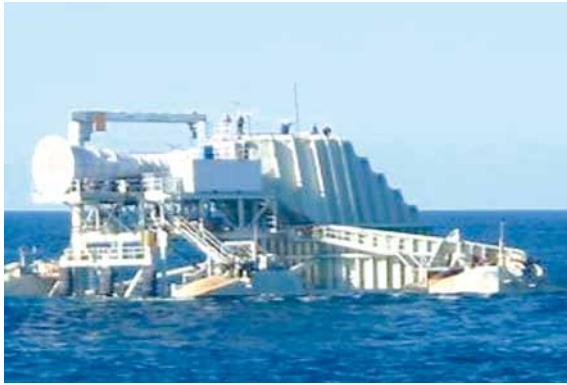
▲ FIGURE 5: Oscillating water column (Courtesy: Oceanlinx)
