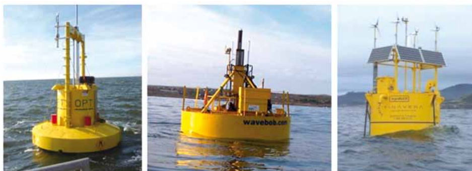
▲ FIGURE 2. Heaving point-absorber prototypes: Powerbuoy, Wavebob and Aquabuoy.
