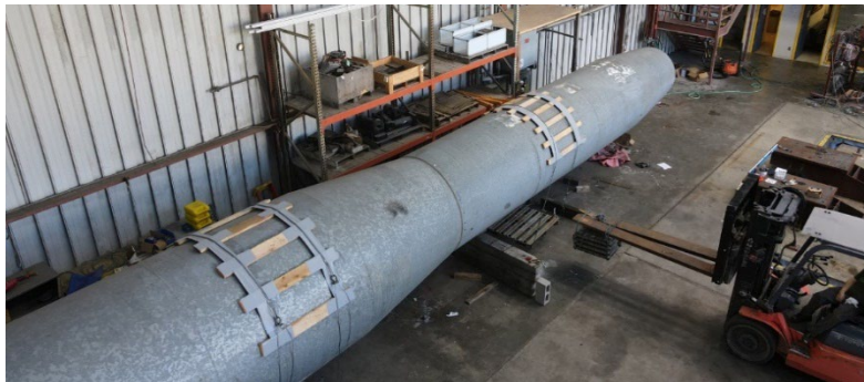
Figure 2: Turbine Being Loaded With Weights During the 4-Point Bend Test
