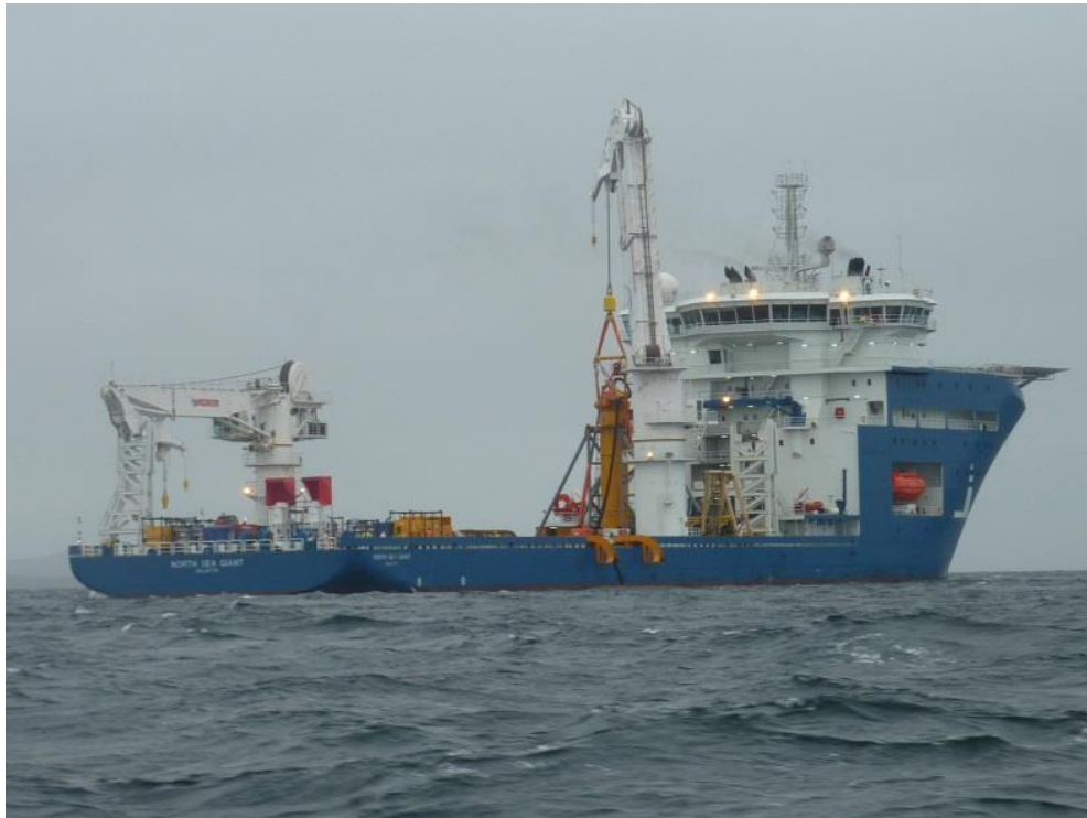
Figure 19.6: North Sea Giant DP vessel installing foundation Voith turbine
