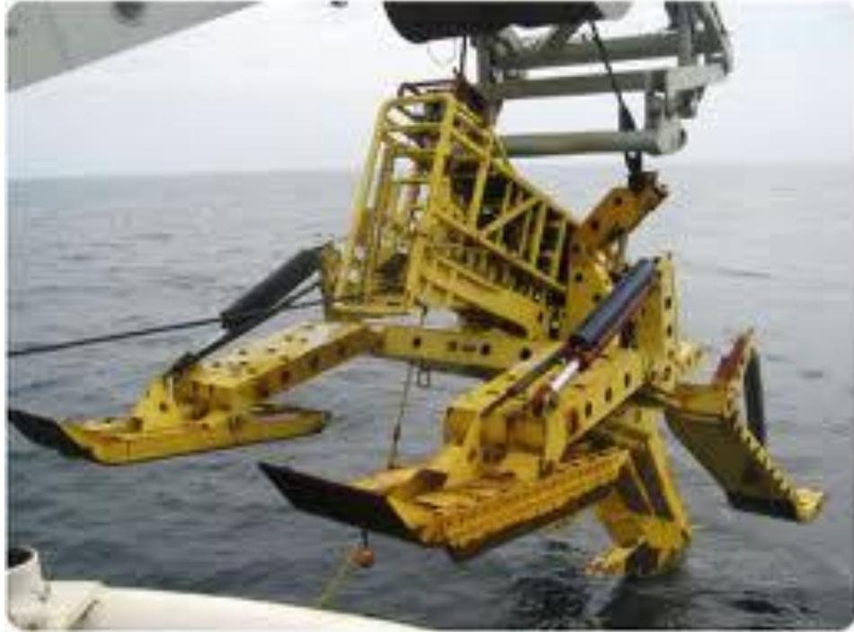
Figure 5.25: Plough for Shallow Waters and Intertidal Zone
