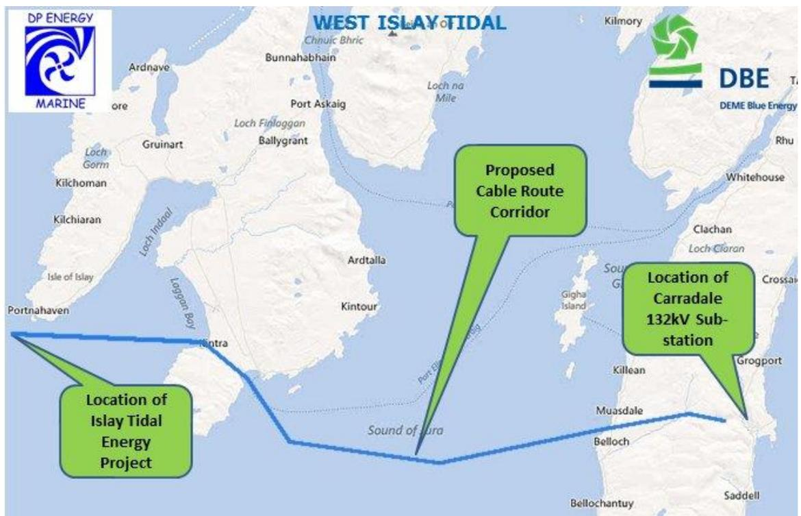
Figure 5.2: Proposed Grid Connection Cable Route (For Information Only)
