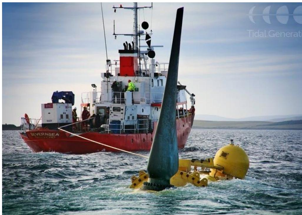
Figure 5.31: O&M Vessel Towing TGL Device
