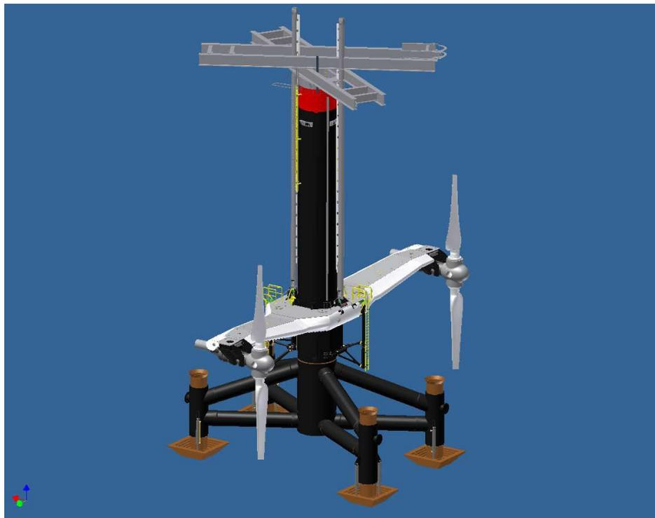
Figure 5.14: Quadrapod Foundation Illustrating Temporary Top Beams
