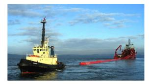
Figure 2.28 Pelamis deployment (source: Ocean Prospect Ltd)
