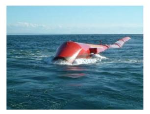
Figure 2.13 Pelamis device (source: Ocean Prospect Ltd)
