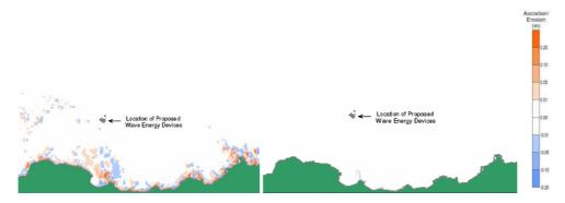
Figure 6.18 (left) and Figure 6.19 (right) Prediction of the effect of the typical case WEC layout on the sediment transport regime with and without the existing wave and current regime respectively
