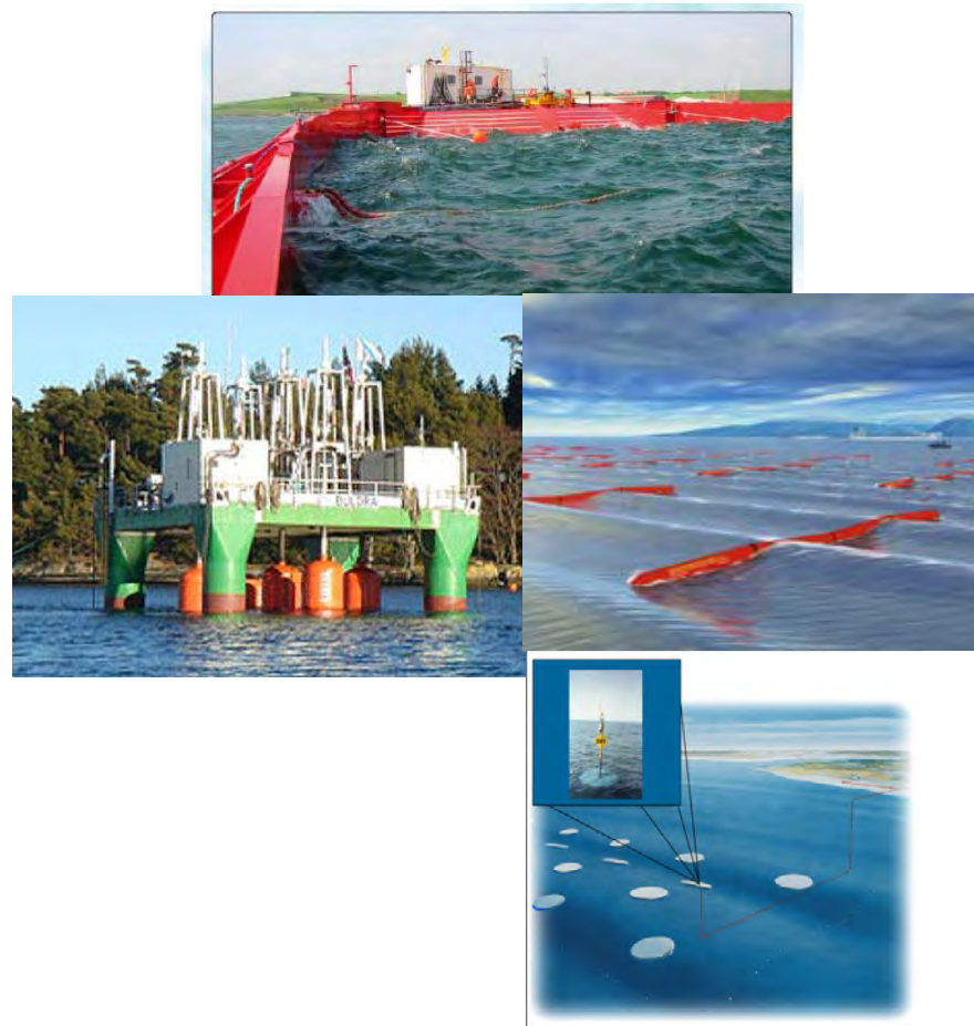
Plate 1.1: WEC Devices (top to bottom: Wave Dragon, FO 3 , Pelamis and PowerBuoy PB150)
