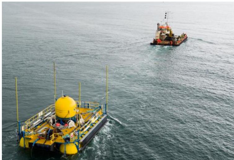
**Figure A8. WaveSub from Marine Power Systems [19]**
