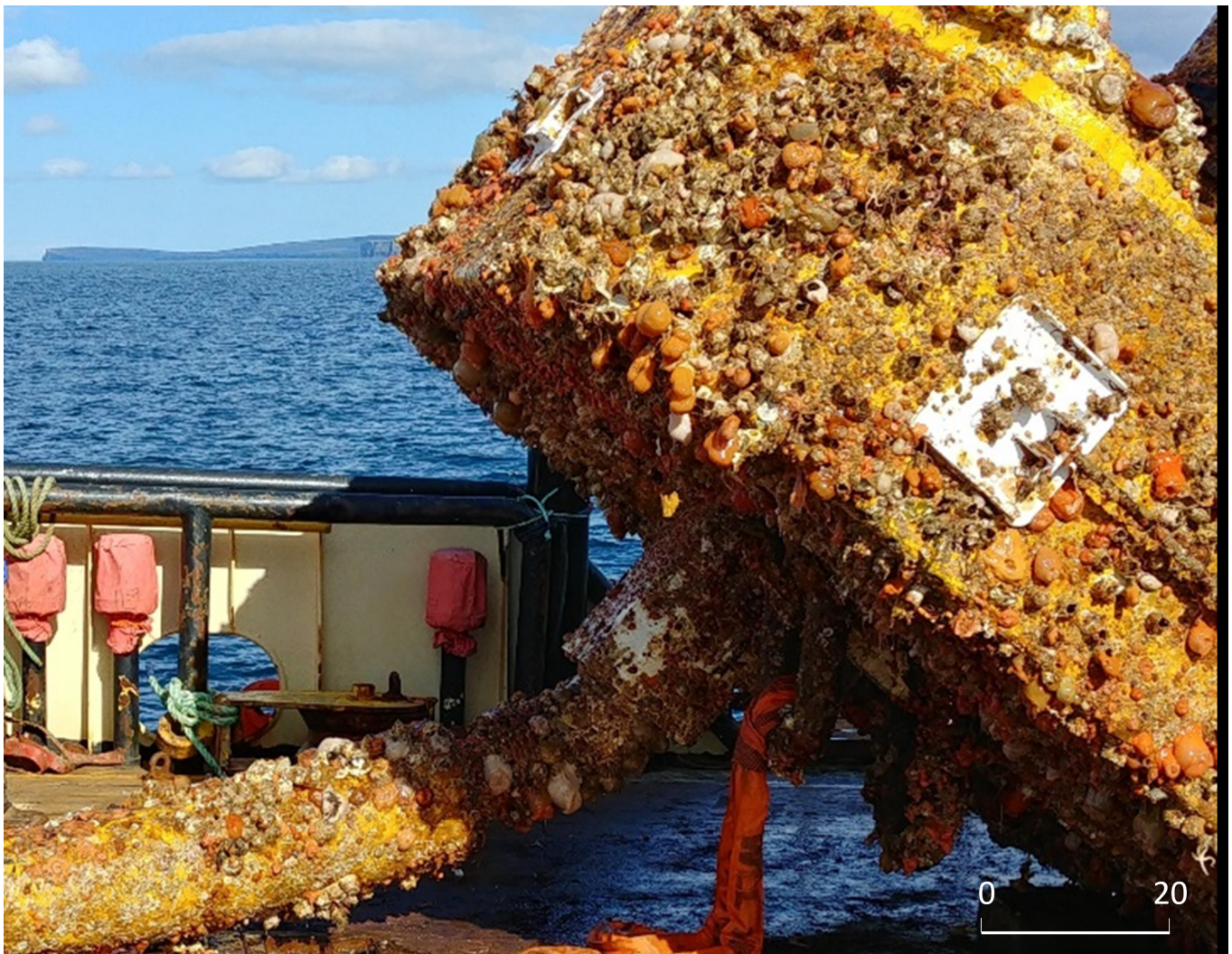
Figure 3. Biofouling of the tether latch assembly (TLA) mooring system of a wave-energy converting device. Scale bar 0–20 cm (image: EMEC).
