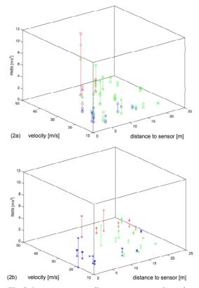
Fig. 2: Impact energy vs. distance to sensor and speed. colors: blue-green-red: increasing mass symbols (2a): □ frontal, O frontal-suction side, symbols (2b): \* grazing, + suction side, x pressure side
