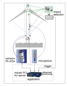
A new monitoring system for registration of bird collisions, WT-BIRD, has been developed at ECN [5]. It uses video cameras and microphones combined with event triggering by sound and vibration measurements. Figure 1 shows a schematic overview of the system.
