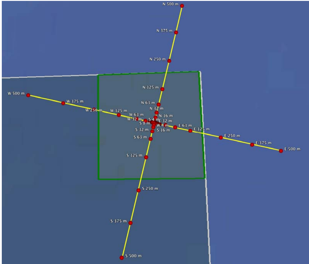
Figure 2. Each seafloor EMF measurement station is shown as a red dot lying along either a N-S or E-W (magnetic coordinates) survey line. Survey locations are found 4m, 8m, 16m, 32m, 63m, 125m, 250m, 375m and 500 m radially outward from the array center, in each of the four cardinal magnetic directions.
