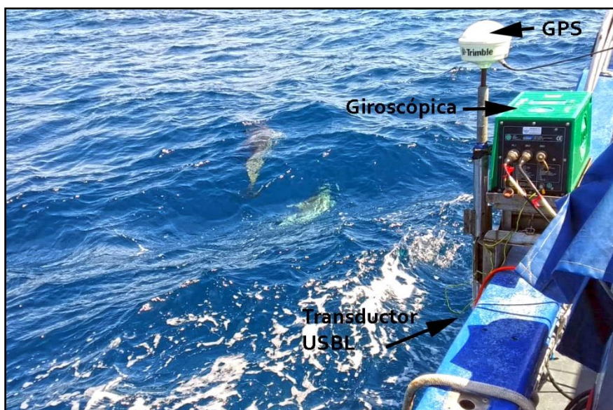
Figure 9. Mounting on the band of the USBL, gyro and GPS.
