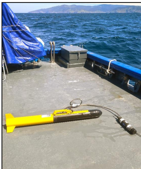
Figure 10. GeoAcoustics 100/500 kHz side-scan SONAR, including a GeoAcoustics transmitter-receiver unit and an underwater location pinger.
