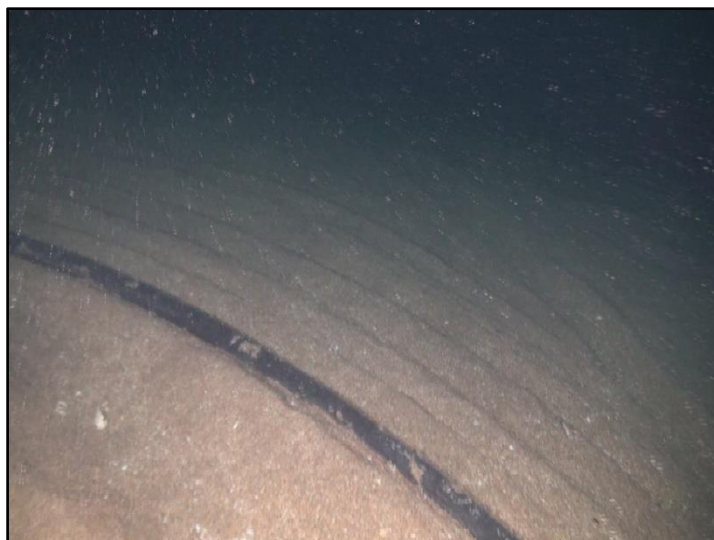
Figure 32. The wire turns roughly 90°. Some footprints at the side of the wire indicate different lines the wire has been placed previously.
