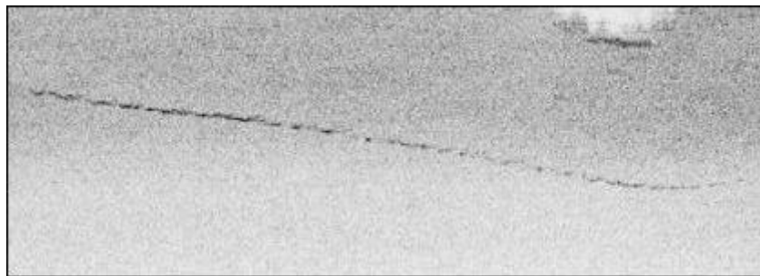
Figure 36. Sonar record (100kHz) where the unearched cable can be seen on a sandy bottom.
