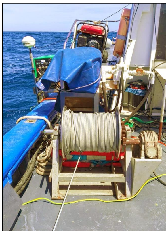
Figure 11. Side-scan SONAR winch and towing cable.
