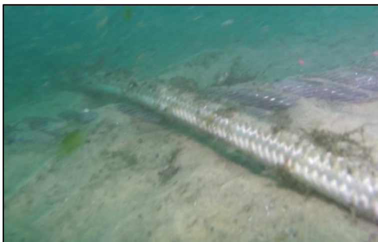
Figure 45. A synthetic mooring cable crossing a steel mooring cable. (GoPro camera).
