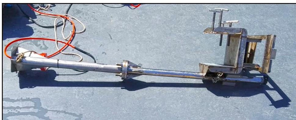
Figure 8. USBL bar mounted transducer to be installed on the band.
