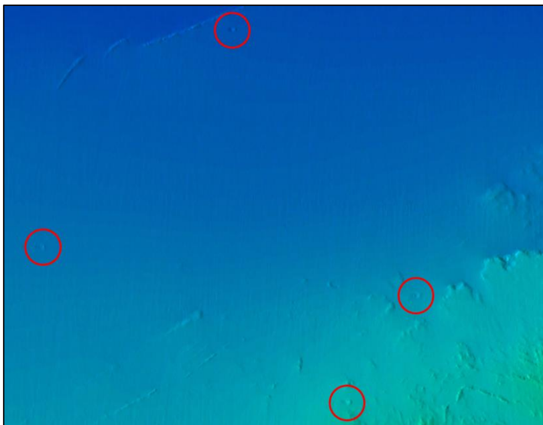
Figure 22. Footprints (inside the red circles) probably caused by the anchoring operation in a bathymetry obtained in September 2017 (the anchoring was carried out in June 2016).
