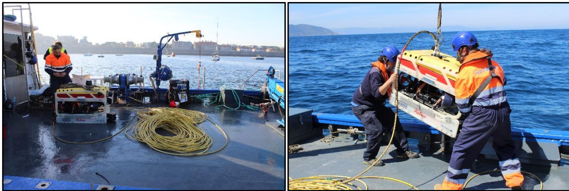
Figure 4. SEAEYE Falcon DR ROV employed in the seafloor monitoring in BiMEP. On the left, all the equipment on board the vessel. On the right, the ROV ready to be deployed in the sea.
