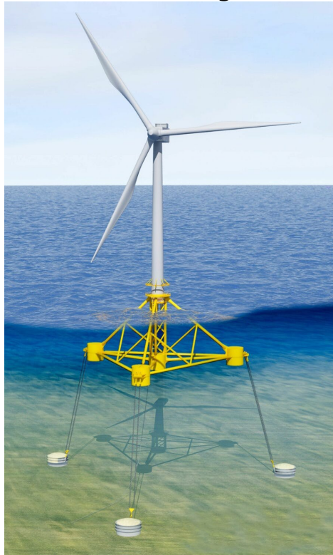
Figure A-5: SBM Tension Leg Platform Concept
