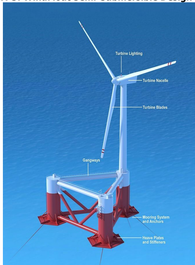
Figure A-3: WindFloat Semi-Submersible Design Concept
