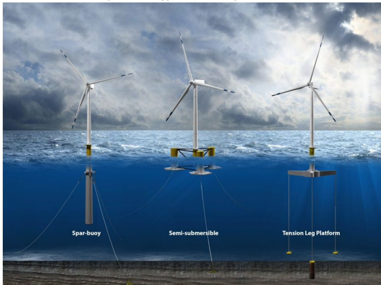
Figure 2-2: Types of Floating Platforms
