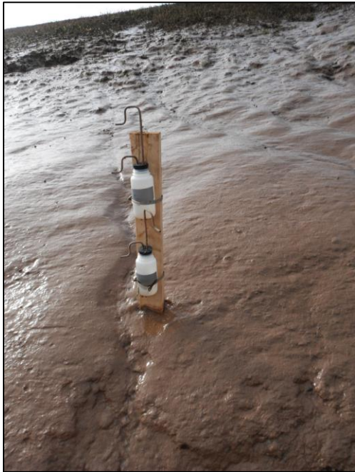
Figure 8: Rising stage bottles deployed at C4 in May 2013.
