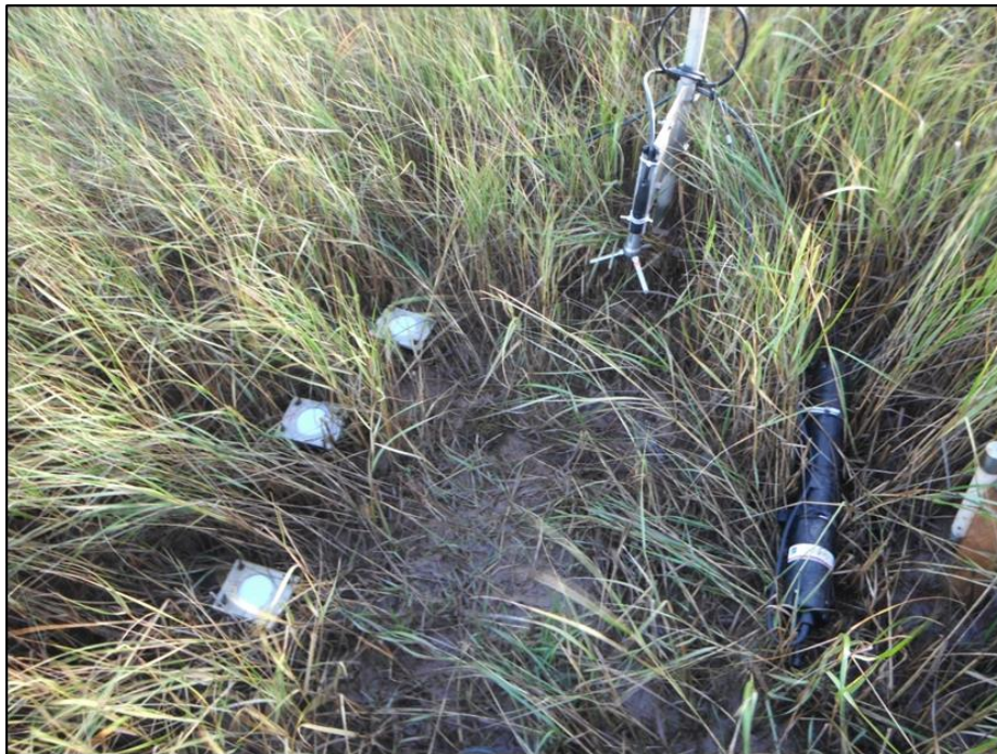
Figure 5: ADV, sediment traps, rising stage sampler and ISCO inlet nozzle at M3 on Sept. 19th, 2012. Note considerable vegetation growth.
