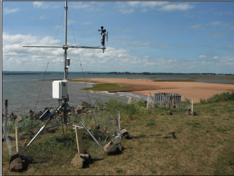
Figure 9: Weather station deployed on a cliff immediately west of the sampling site
