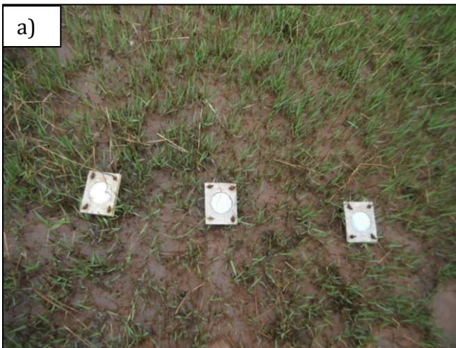
Figure 7: Surface mounted sediment traps deployed at a) M3 prior to the tide on May 25 and b) after the tide at C4 March 27, 2013.
