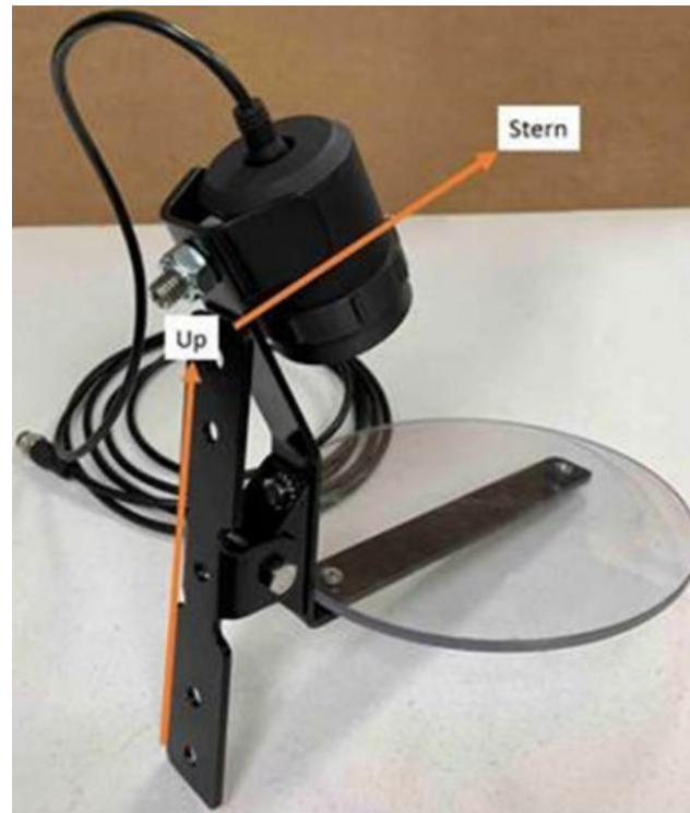
Figure 2. Photograph of Microphone and Reflector Plate Depicting the Correct Orientation of the Device
