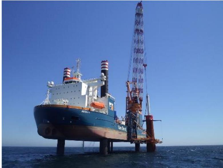
**Figure 3-2. Monopile Installation** *Source: Globalenergyworld.com*
