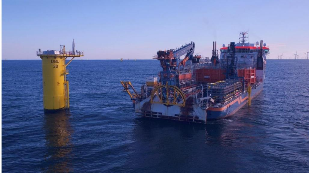
**Figure 3-14. Dynamically Positioned Cable Installation Vessel**
