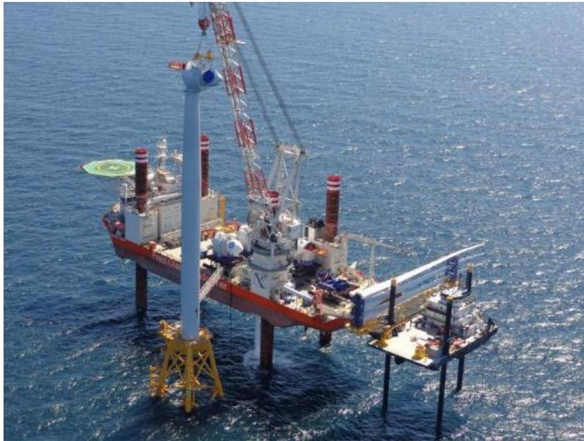
**Figure 3-17. Offshore WTG Installation Vessel** *Source: blockisland.com*
