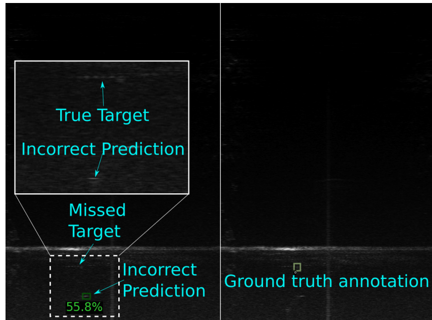
Fig 2.3.6. Example failure case #1 at Grand Passage. Right: Ground truth target. Left: Predicted target, which is not in the correct location. As an incorrect target is found, and a false positive is recorded. If using IoU recall (sec 2.3.2.3), a false negative is also recorded since the pixel location of the predicted target is incorrect. If using frame recall, a false negative is not recorded, as a detection occurred, just in the wrong location.
