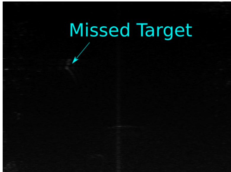
Fig 3.2.4. Example failure case #1 at Grand Passage. Target (V-Wing) missed by detector. This was a rare case, but did occur at times.
