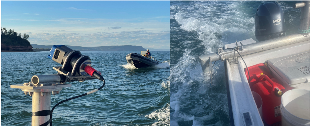
Figure 2.1.10: Pole-mounted Gemini on research vessel Puffin
