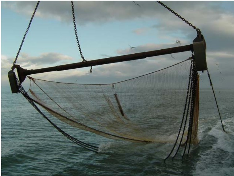
Photo 2. One of the 6m beam trawls used on board the research vessel 'Isis' during the Baseline surveys. Attached to this beam is the 20 mm net. In the middle of the net, the CTD device is visible.
