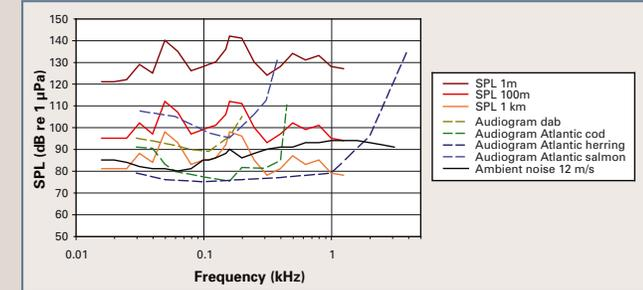
Figure 3: Attenuation of operational noise at different distances from the source, ambient noise levels and audiograms of target fish species (operational noise after ITAP (2005); values as dB<sub>rms</sub> re 1 µPa in 1/3 octave-bands; TL-calculations after Thiele (2002); background noise levels in 1/3 octave-bands in dB<sub>rms</sub> re 1 µPa after Betke et al. (2004); audiograms after Enger 1967; Chapman and Hawkins 1973; Chapman and Sand 1974; Hawkins and Johnstone 1978).
