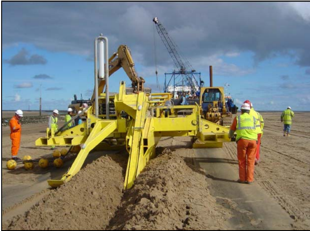
Figure 2.7 Example of plough used to install offshore cables
