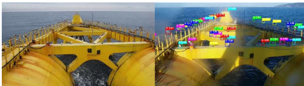
Figure 10. Photos of AI-powered bird monitoring at the DemoSATH floating wind platform. Source: Saitec Offshore Technologies.
