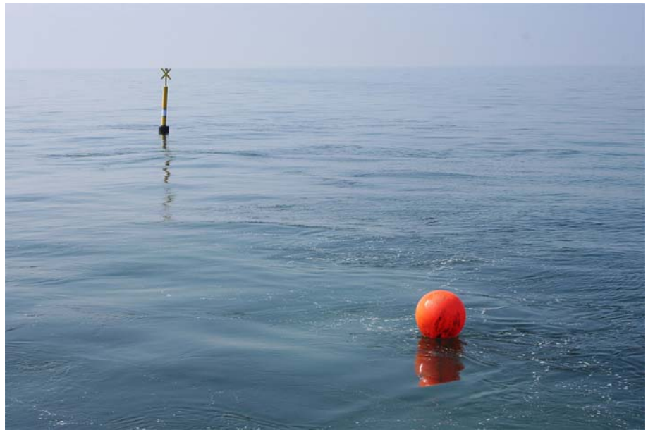
Figure 2.8. The buoy system seen from the surface. The red float is used to retrieve the instruments without pulling the heavy anchor up.
