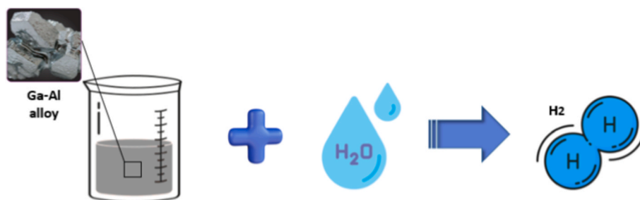
Fig. 18. Generating hydrogen through water splitting using a Ga-Al composite, reproduced with permission from Ref. [188].
