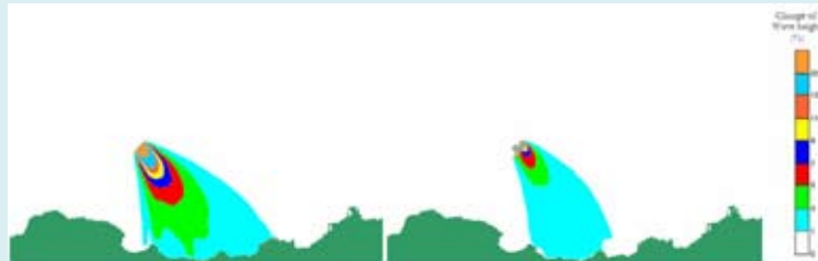
Figure 9.1 Worst case scenario layout, 1 in 1 year storm event conditions ( H_s = 10\text{m} , T = 12\text{s} ) (left) and typical case scenario layout, 1 in 1 year storm event conditions ( H_s = 10\text{m} , T = 12\text{s} ) (right)
