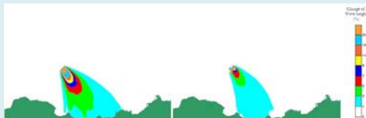
Figure 9.2 Worst case scenario layout, small wave conditions ( H_s = 1\text{m} , T = 7\text{s} ) (left) and worst case scenario layout, large wave conditions ( H_s = 4\text{m} , T = 16\text{s} ) (right)
