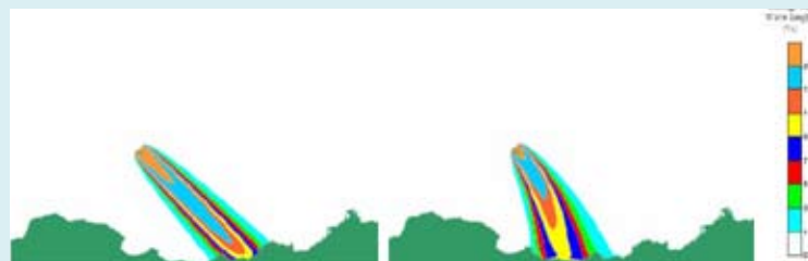
Figure 9.3 Worst case scenario layout, small wave conditions ( H_s = 1\text{m} , T = 7\text{s} ) (left) and typical case scenario layout, large wave conditions ( H_s = 4\text{m} , T = 16\text{s} ) (right)
