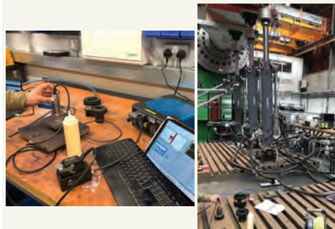
Figure 4: EXPERIMENTAL SETUP FOR PAUT (M36 LEFT, M42 RIGHT)
