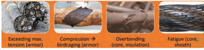
Fig 2: Power cable failures (Manuel Rentschler, WavEC Annual Seminar)
