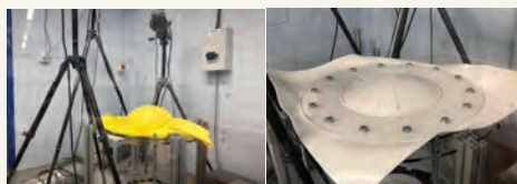
FIGURE 2: The experimental setup of the bulge test
