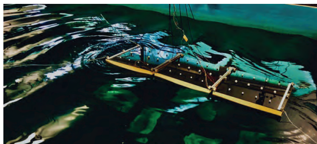
Figure 1. Laboratory scale very large hinged floating structure tested in the Kelvin Hydrodynamics Laboratory at the University of Strathclyde under regular waves
