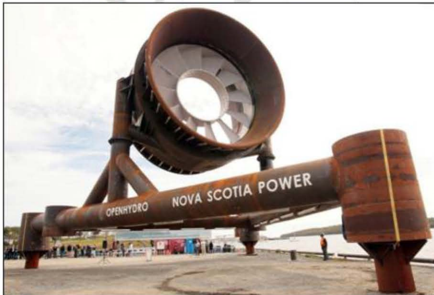
FIGURE 2-3 TRIAL ASSEMBLY OF 10 METER OPENHYDRO TURBINE & SUBSEA BASE (DARTMOUTH, NOVA SCOTIA, CANADA)
