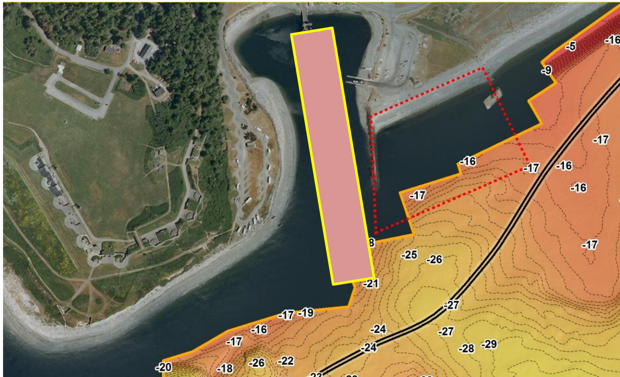
Figure 1. March 2012 dredged zone for Keystone Harbor (rectangle). Dredged area ends well north of cable run.
