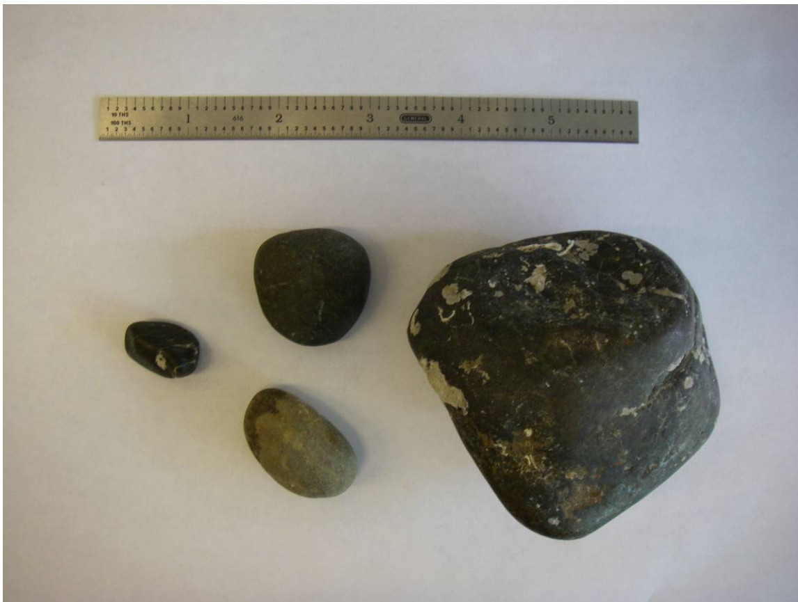
FIGURE 3-3 NNMREC GRAB SAMPLES IN THE TURBINE DEPLOYMENT AREA
