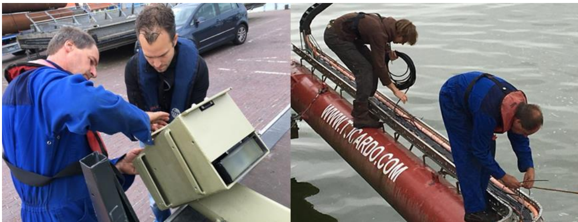
Figure 7.2: Installing the DIDSON in the housing (left) and fixing the DIDSON cable to the beam structure in sluice 2.
