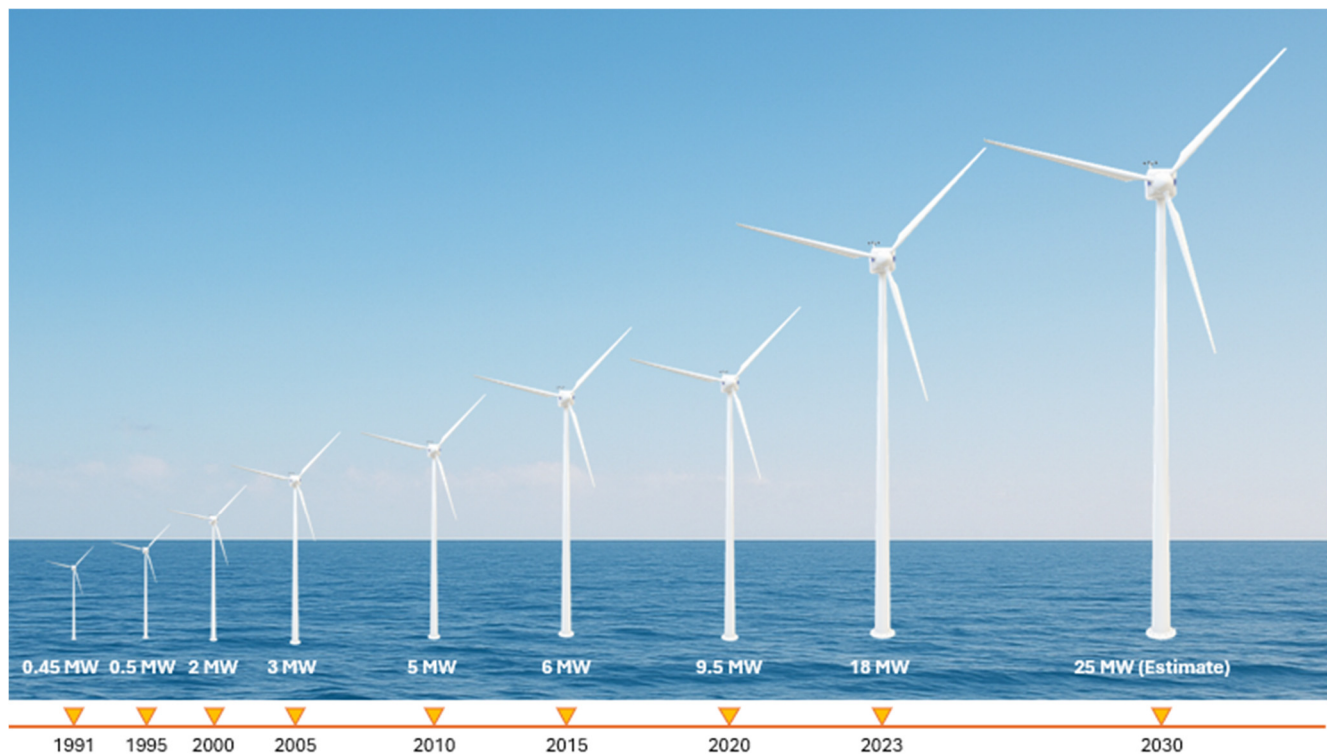
Figure 7. Offshore wind turbine capacity evolution. Adapted from [84].
